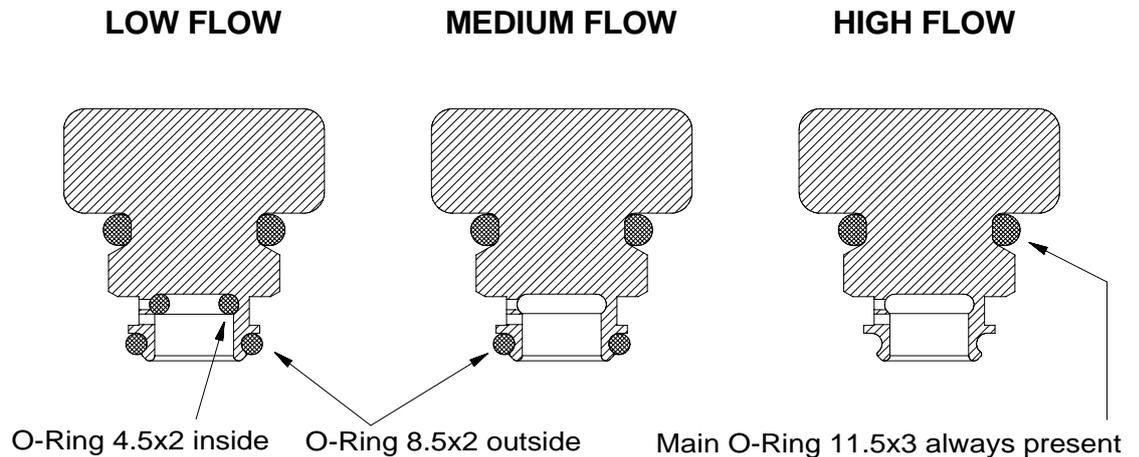
**NB:** The flow rate should be checked on both, the clean water supply and the separator sample supply. If the clean water supply is obtained from a high pressure source, the flow rate will be higher than from the sample point.
